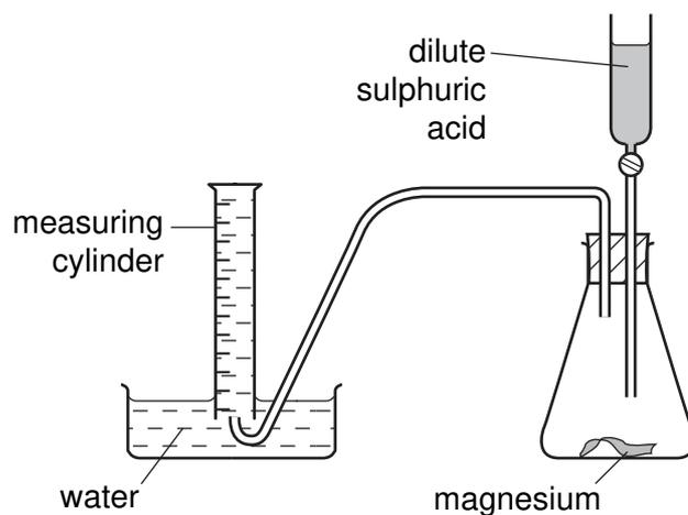
In an experiment  $50 \text{ cm}^3$  of dilute sulphuric acid was added to a large piece of magnesium. A student measured the total volume of gas produced at 2 minute intervals.
